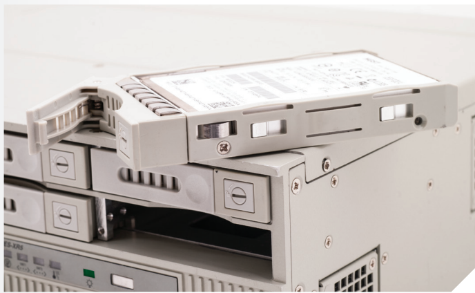
Eight Removable, Hot Swappable, Front Access Drives
