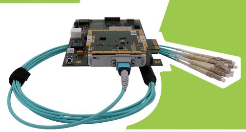
Optical communications have become the new standard in the embedded industry with the increasing demand for bandwidth. This demand is driven by new high-resolution sensors and by intercommunications needed among processing units.
