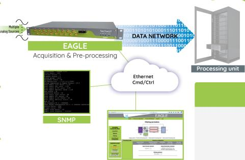
EAGLE is an unique solution which allows to manage multi-channels acquisition and to offload data pre-processing stages from real-time calculators. EAGLE shares the processed data with the communication network making this acquisition solution highly-scalable.
